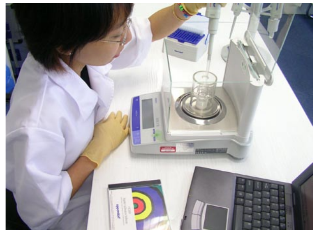
Fig. 4: Pipette calibration using an analytical balance with moisture trap
